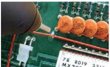
Product assembly with a slim profile to help operators apply adhesive more accurately.
