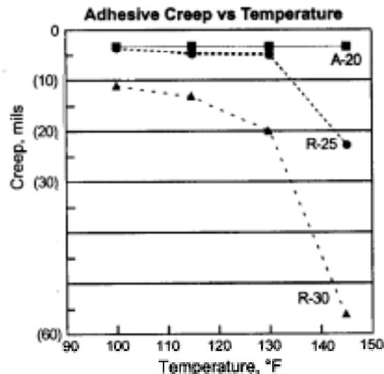
3M Test Method – Inclined Plane Static Shear Test Method; 30° incline, tested on ABS using ½ inch diameter die cuts from SJ-5816, SJ-6016 and SJ-6216 Rollstock products. 2 lb. Load per ½ inch diameter die cut. Measured time of creep: 15 minutes.
