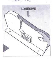
Load the adhesive tape on the core.
